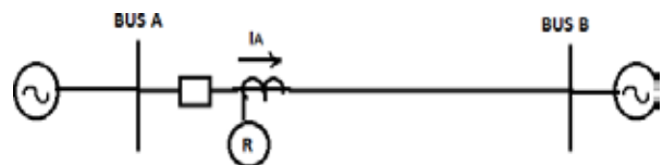
Fig. 3 Basic principle of distance protection
